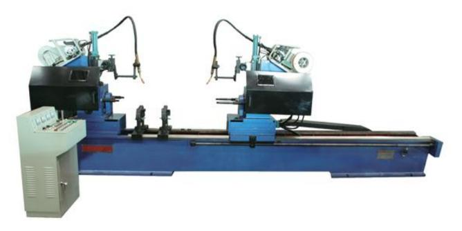
Conveyor Idler Roller manufacturing process involves various sub-processes, one of them is the welding of the bearing housing to the cut-off pipe on both ends after the pipe is bevelled and boring is done at both the ends. This can be done by manually or by mechanized / automated systems. Improper welding in this stage may affect the quality of the end product i.e. finished idler roller.
