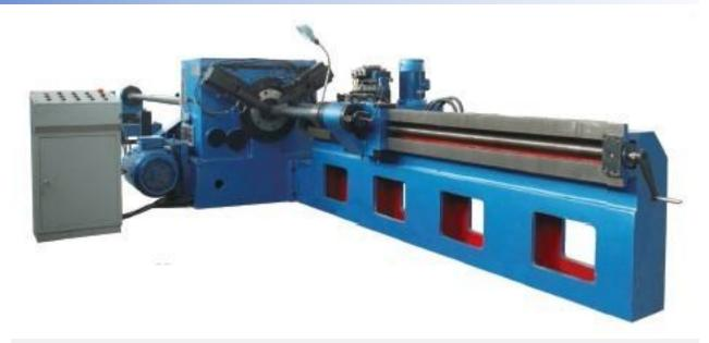
This is an automatic system for fixed-length cutting of steel pipes for manufacturing idler rollers. The cutting and bevelling of pipe is done simultaneously. The cutting tool head is fixed while the tool is fed by hydraulic cylinder and pipe rotates at high rpm, which delivers high cut quality with precision.
