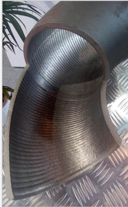
Cut-sectional view of Elbow ID after Cladding
